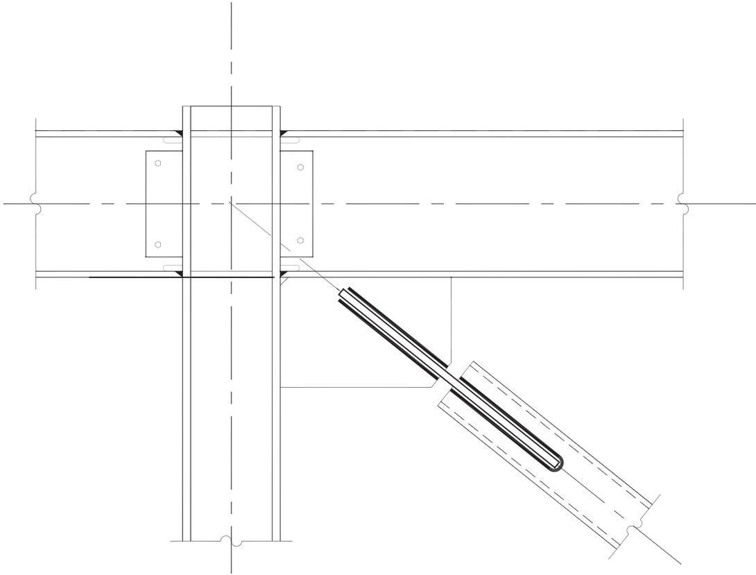
Figure 2-3. Typical gusset configuration
